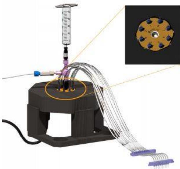
Connect the pump, from its output port to either the centre of the MultiFlow8 or to the 3-way adapter, depending on the Multiflow8 setup. With all valves open, run the 'dispense reagents' step several times to wash through all ports of the MultiFlow8.
